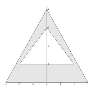
This trivial example has the obvious solution  $\phi = 1$  throughout the domain. However it provides a useful illustration of data input for a doubly-connected domain. The solution is computed at one corner of each triangle and at one point inside the domain.
