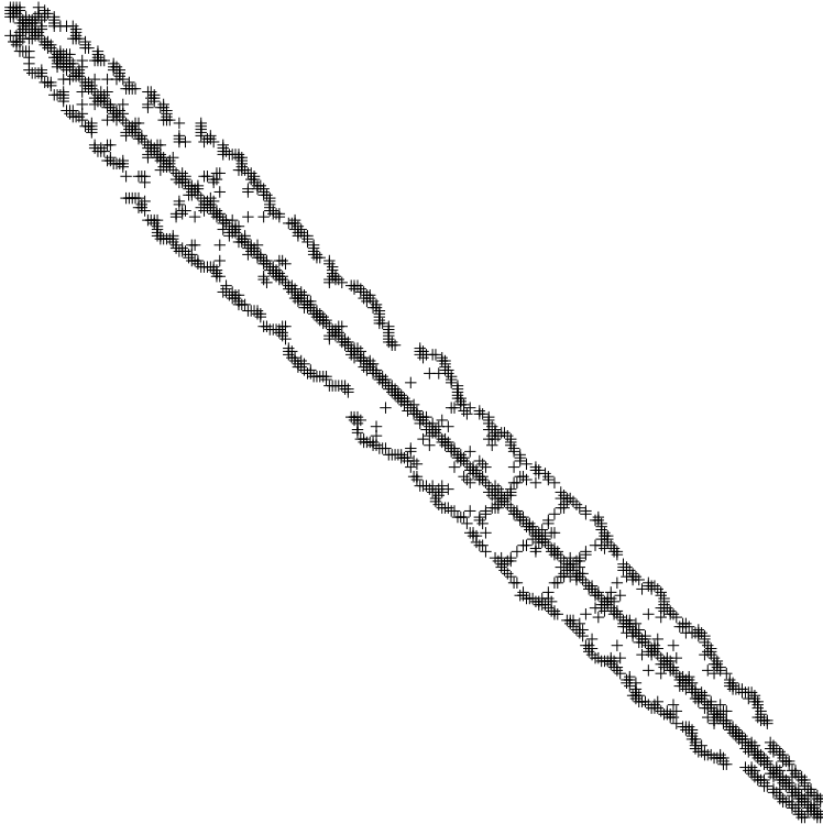
Figure 3: Sparsity of the FE Matrix After Renumbering
